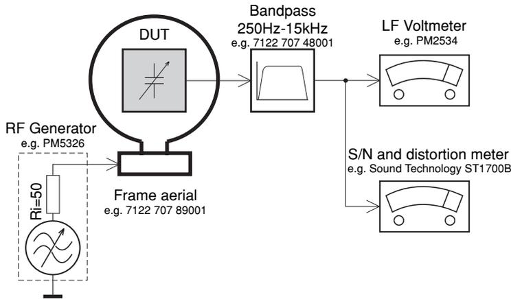
To avoid atmospheric interference all AM-measurements have to be carried out in a Faraday«s cage. Use a bandpass filter (or at least a high pass filter with 250kHz) to eliminate hum (50Hz, 100Hz).
