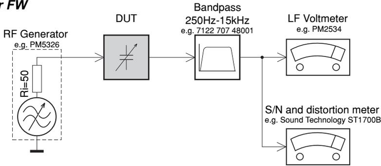
Use a bandpass filter to eliminate hum (50Hz, 100Hz) and disturbance from the pilotone (19kHz, 38kHz).
