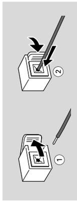
Fully insert the stripped portion of the speaker wire into the terminal as shown.
